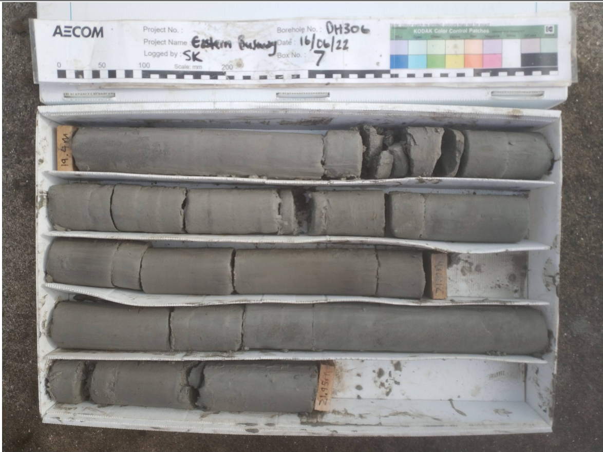
Box: 7 of 9 - Depth: 19.40m to 21.95m of 25.50m Date Drilled 15/06/2022 to 16/06/2022 - Date Photographed: 16/06/2022
