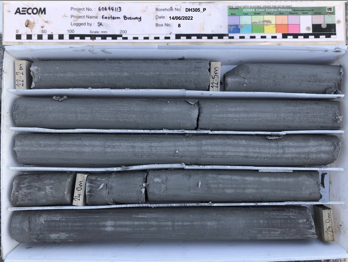
Box: 8 of 10 - Depth: 22.20m to 25.00m of 30.00m Date Drilled 13/06/2022 to 15/06/2022 - Date Photographed: 14/06/2022
