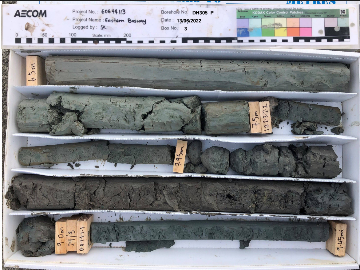
Box: 3 of 10 - Depth: 06.50m to 09.45m of 30.00m Date Drilled 13/06/2022 to 15/06/2022 - Date Photographed: 13/06/2022
