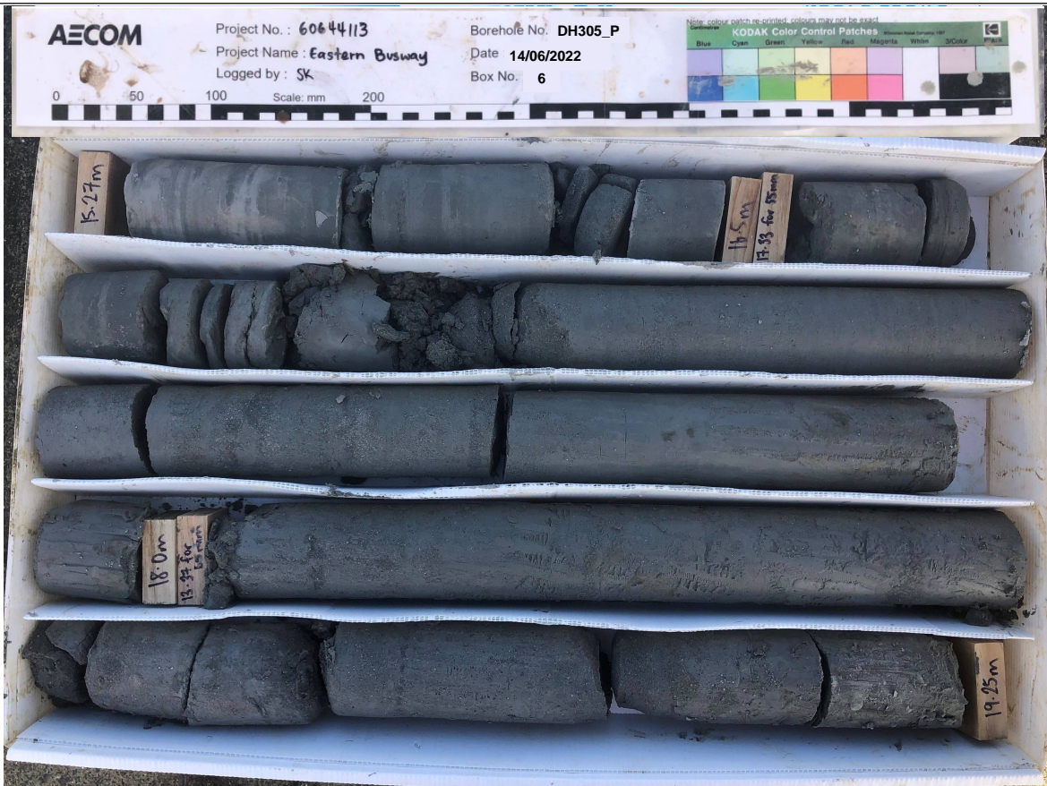
Box: 6 of 10 - Depth: 15.27m to 19.25m of 30.00m Date Drilled 13/06/2022 to 15/06/2022 - Date Photographed: 14/06/2022
